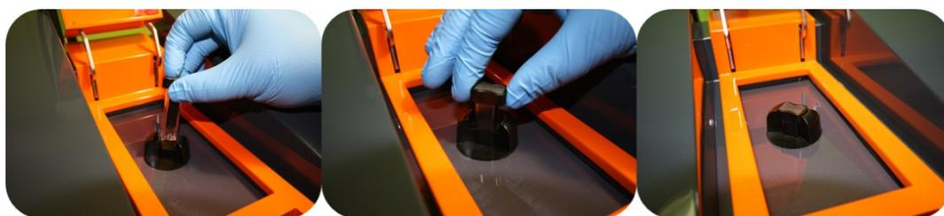
Figure 11: How to insert electrodes head and cell in cell holder (photos)
