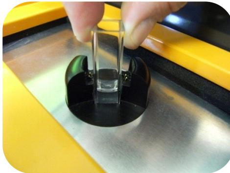
Figure 4: Insertion of cell in cell holder
