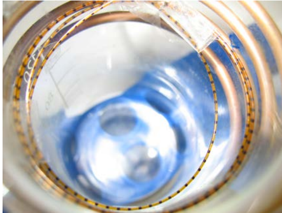
Fig. 4. Microfluidic train of magnetic droplets in a thermally insulating oil to confine the heat produced by RF hyperthermia. Here the flow-rates Q_2/Q_3 are respectively 50/150 \mu\text{L} \cdot \text{min}^{-1} thus the magnetic fluid occupies Q_{\text{MF}} = 25\% v/v.
